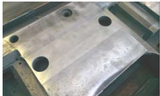
The Laser clad coating can be machined or ground back to an excellent finish.
