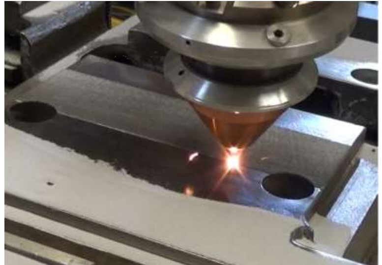
Laser Cladding to repair a cast iron machine table
