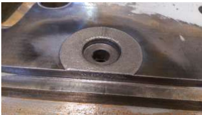
Laser Cladding can be accurately applied to repair localised areas.
